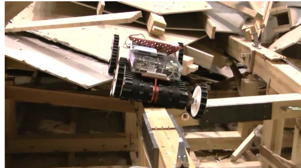
Mobility on beams of roof
