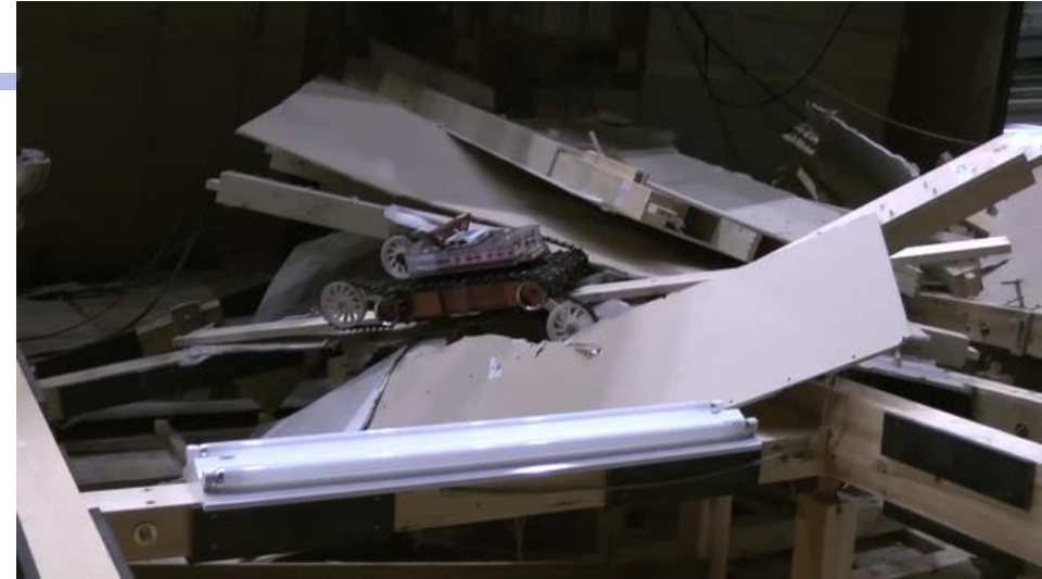
Mobility at collapsed roof
