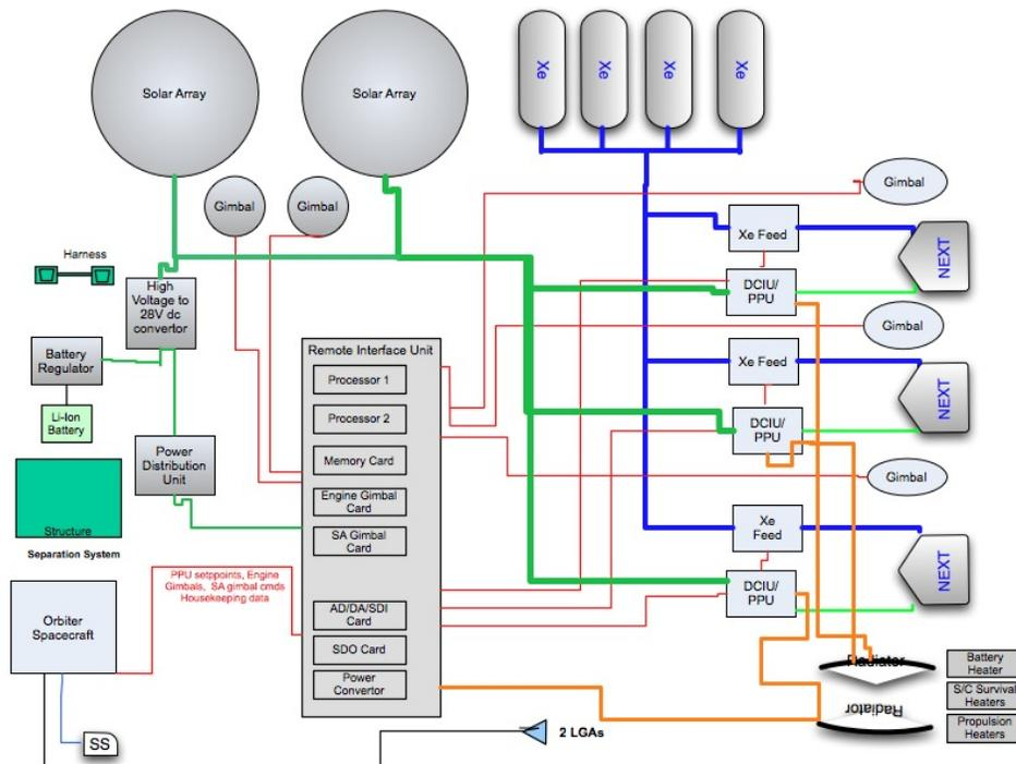
**Figure 3-2. SEP stage block diagram.**
