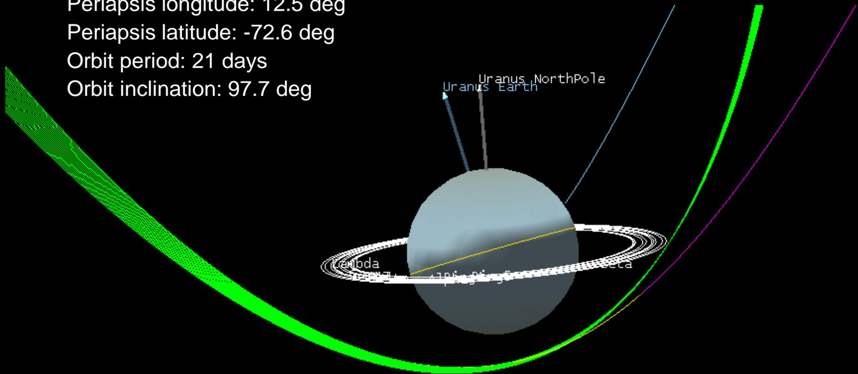
20 highly inclined elliptical orbits providing the desired science measurements (atmosphere, magnetic field, gravity field)
