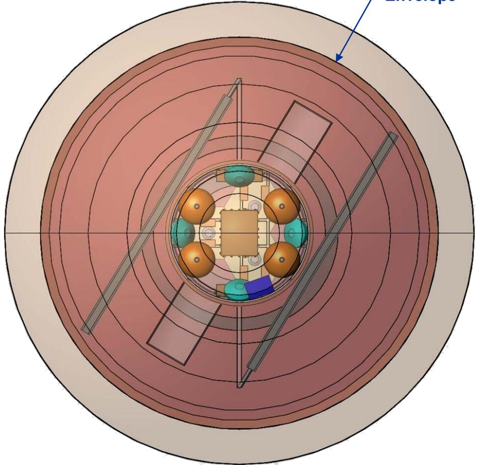
4.58 m Diameter Static Payload Envelope
