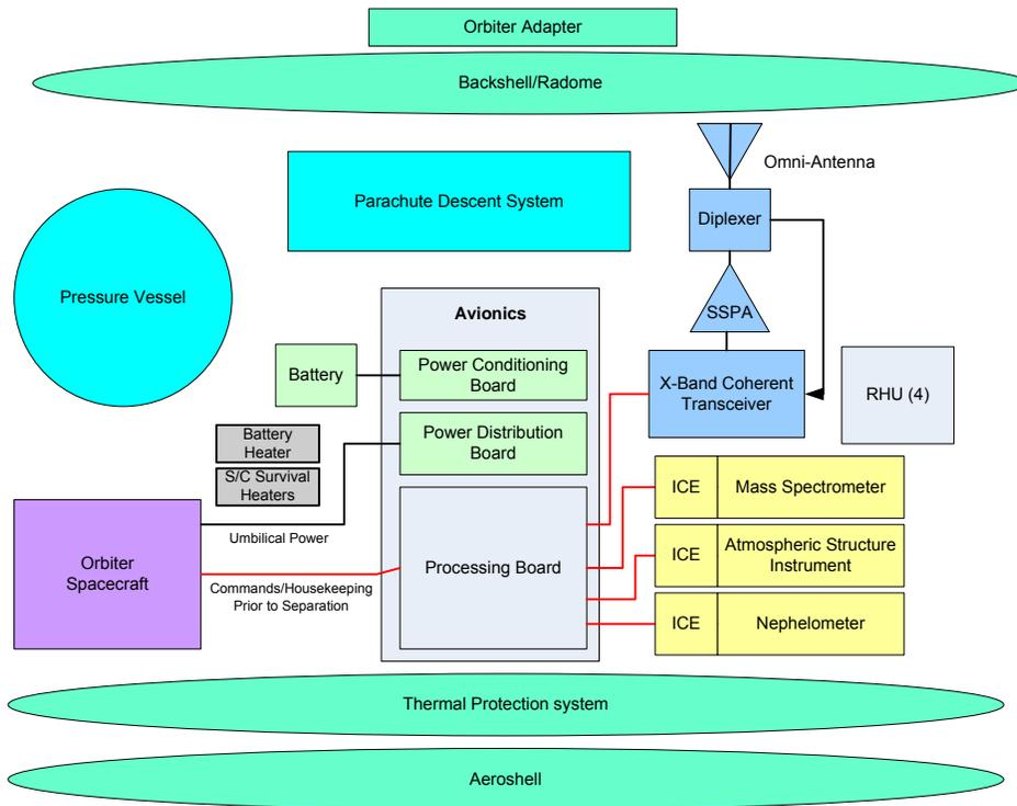
**Figure 3-6. Entry probe block diagram.**
