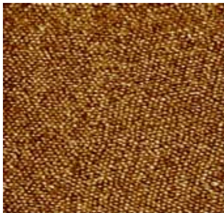
Fig. 1. (A) AFM image of P(S-b-MMA) copolymer film with cylinders oriented normal to the surface. Each cylinder is \sim 13 nm in diameter.
