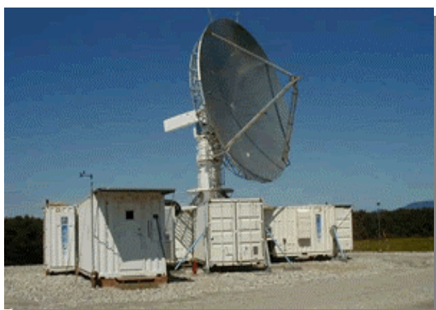
S-POL Radar (NCAR) – its modularity allows for reasonably easy breakdown and set up. Courtesy NSF/NCAR.
