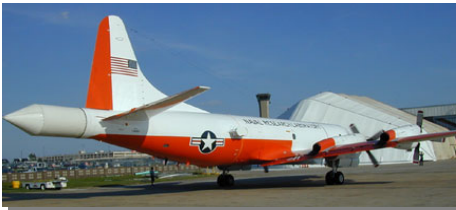
Naval Research Laboratory P-3 with the ELDORA Doppler radar attached to the tail. The P-3 airframe is the only airframe that could be modified to hold the ELDORA. Courtesy NSF's Division of Atmospheric Sciences.
