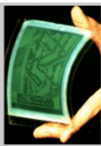
Figure 1: (above) The LCI has created a 200 dpi cholesteric liquid crystal display that could be used in future portable reading devices.
