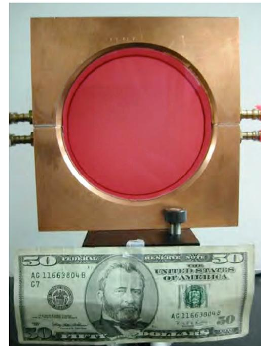
Gain bandwidth in Ti:sapphire is very large → amplification of pulses as short as 20 fs
