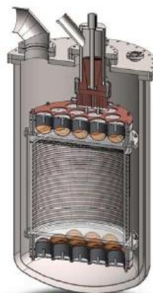
FIG. 5: (a) The DARKSIDE-50 internal detector. (b) The DARKSIDE-50 detector within the active liquid scintillator neutron veto and the passive shield.
