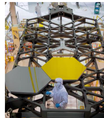
Pathfinder (backplane center section with secondary mirror structure)
