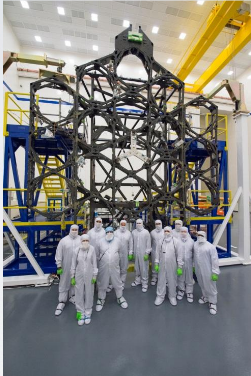
Backplane Center Section and Wings assembled at NGAS
