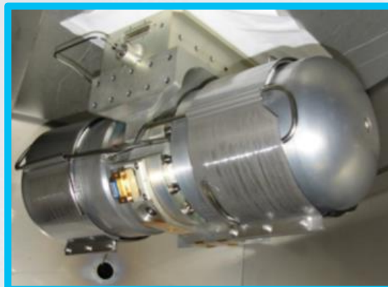
PT Compressor with Interface Plate And Inertance lines installed
