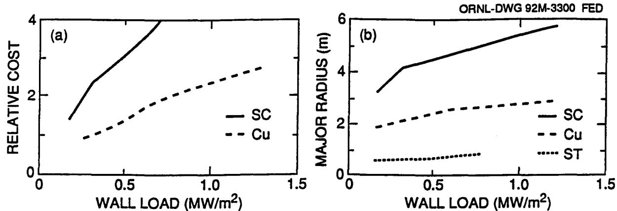
Fig. 1. (a) Minimum cost of Pilot Plants vs. wall load, and (b) the associated major radius. Cases are shown for copper coil (CU), superconducting coil (SC) and low aspect ratio small tokamak (ST), devices.
