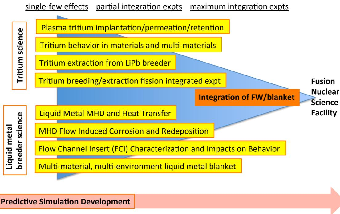
Figure 4. Schematic of the highest priority pre-FNSF R&D program elements in the tritium science and liquid metal breeder science areas, converging into the integrated blanket science.
