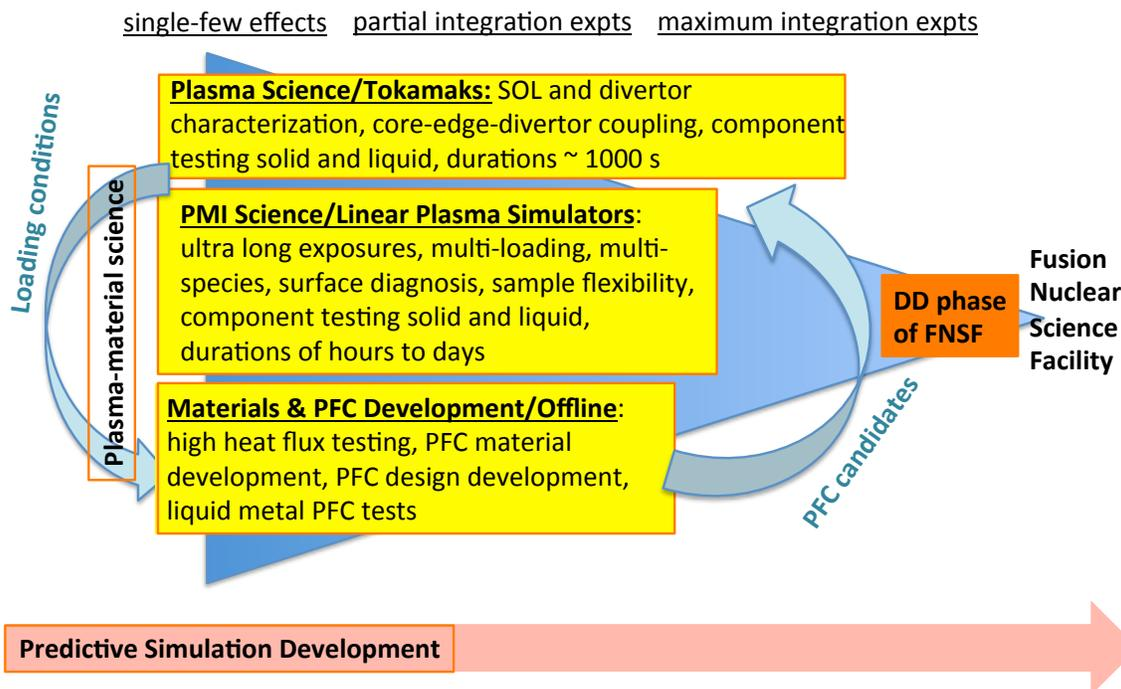
Figure 5. A schematic showing the PMI/PFC pre-FNSF R&D, culminating in the DD phase of the FNSF where ultra-long plasma pulses are created. The interplay between tokamak and linear plasma facilities in providing the testing environments for materials and PFC components is critical for successful development of solutions for a FNSF.
