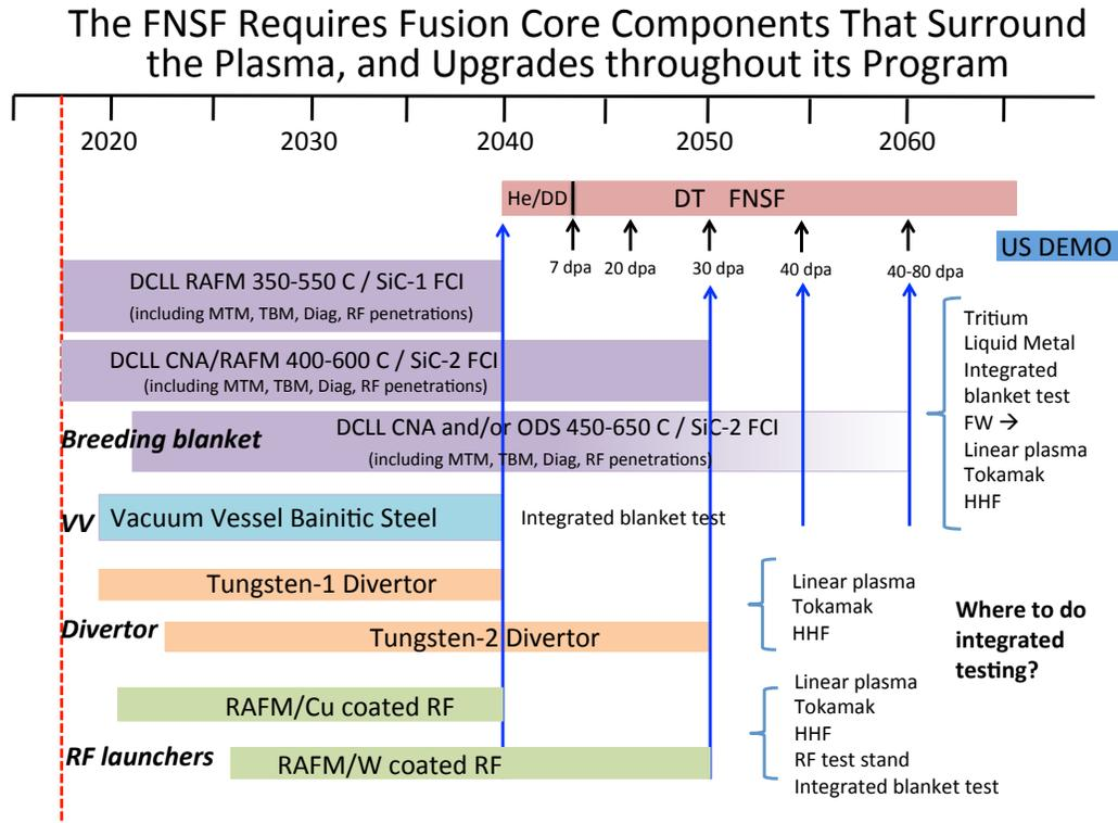
Figure 3. A time-frame showing how fusion core components for the DCLL blanket require development time in order to arrive at the FNSF as industrially produced articles, with the required qualification of fusion relevant neutron exposure and integrated non-nuclear testing of components.
