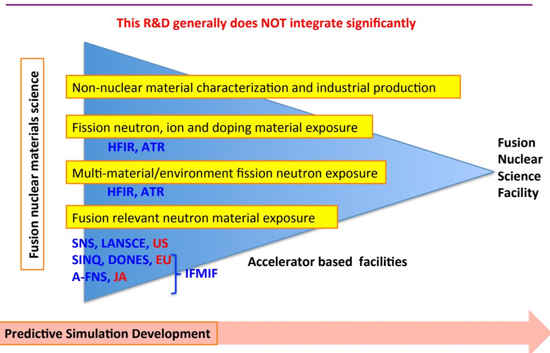
Figure. 2. A schematic description of the major fusion nuclear material elements, highlighting non-nuclear, fission nuclear, multi-material, and fusion relevant nuclear testing. It is difficult to combine this individual material testing with other more integrated testing described later.
