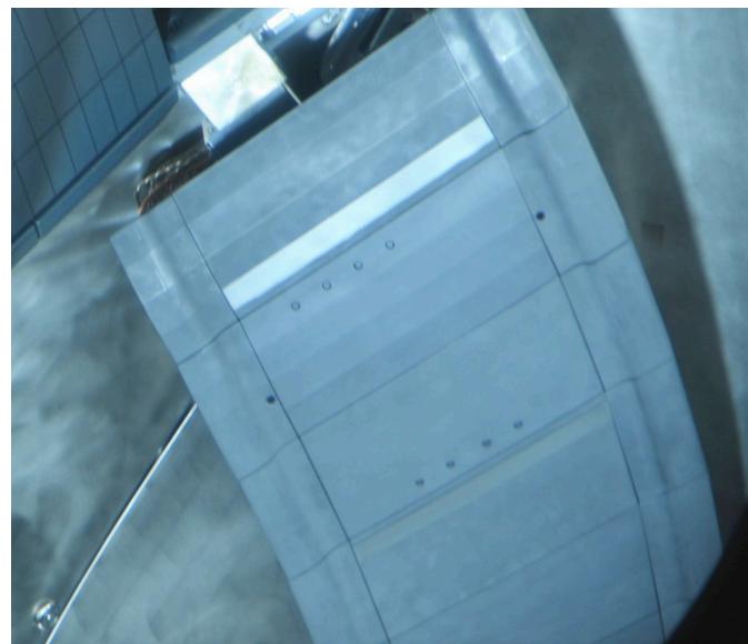
IR camera view of scraper element installed in W7-X
