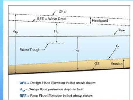
The HPBRS raises the elevation of the lowest floor and horizontal support members to the design flood elevation for the location where the building is sited, or 3 feet above the base flood elevation or the 500 year flood elevation, if known. The end result is that more buildings will be required to use durable foundation systems to support the floors above in areas prone to flooding.
