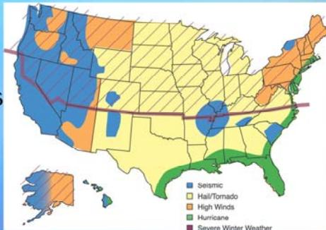
The 2009 IBC includes a new reference to the recently developed ICC Standard for construction of storm shelters. This standard tells someone how to build an effective storm shelter in high wind regions. High wind events include hurricane regions like the Atlantic and Gulf coasts and the interior regions of the country for tornados. The map for tornado regions is different than the design wind speed map in the IBC.
