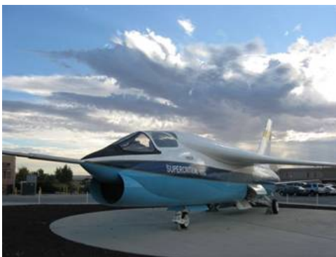
A modified F-8 fighter used for NASA's Supercritical Wing project. The aircraft is one of a number of retired flight test aircraft now located at the entrance to Dryden on Edwards Air Force Base.
