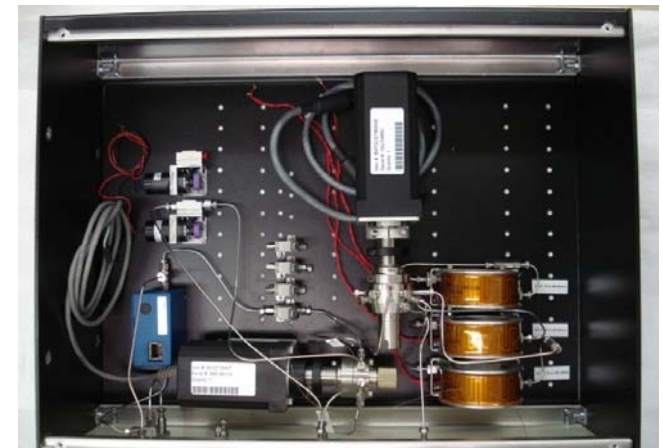
Water Sampling for Front End of Mass Spectrometer for Water Monitoring
