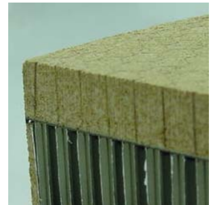
SLA Heatshield Cross-Section (TPS+Struct)
