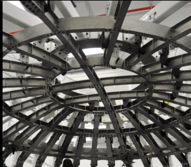
Heatshield Skeleton Assembly at Lockheed Martin in Denver
