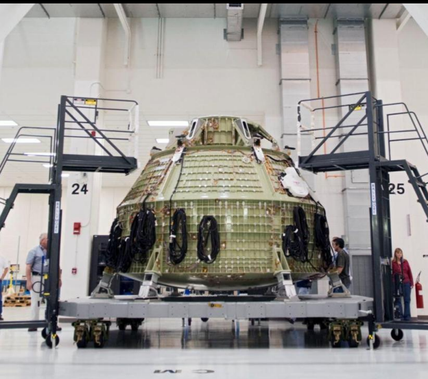
EFT1 Crew Module being moved into the Birdcage tool at the Operations and Checkout Building
