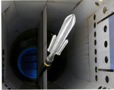
Systems Engineering and Integration SLS model undergoes wind tunnel testing at Langley Research Center (Nov 2012)
