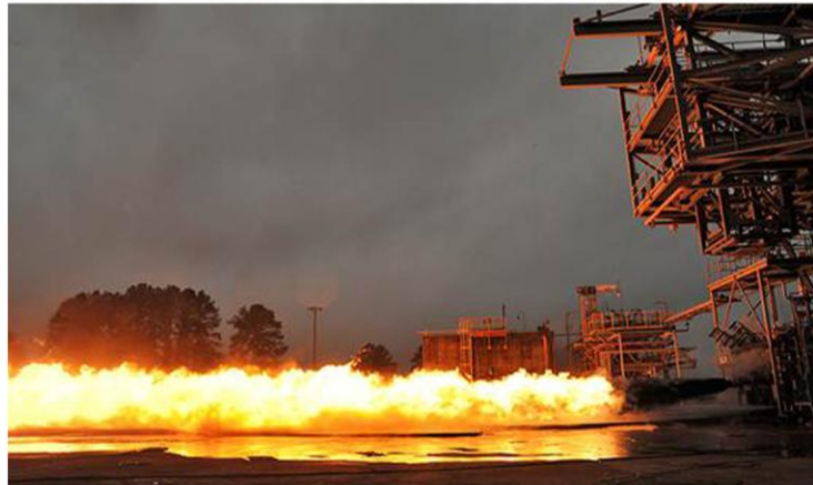
F-1 engine gas generator hot fire test at Marshall Space Flight Center, Jan 2013 – technology development for an optional Advanced Booster concept
