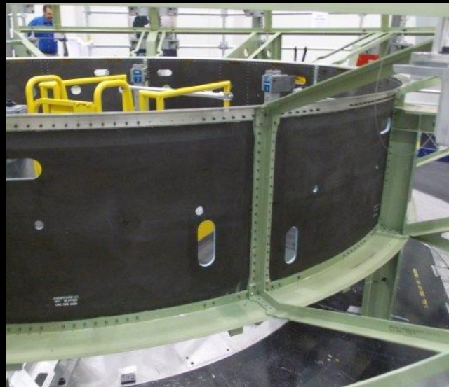
EFT1 Service Module panels being assembled at the Operations and Checkout Building
