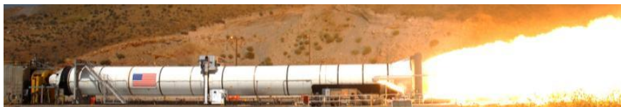
Solid Rocket Booster development motor test in Promontory, Utah, Sep 2011
