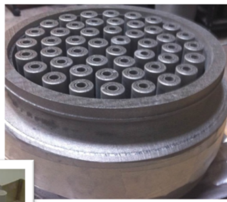
One-piece Injector Built Using Additive Manufacturing
