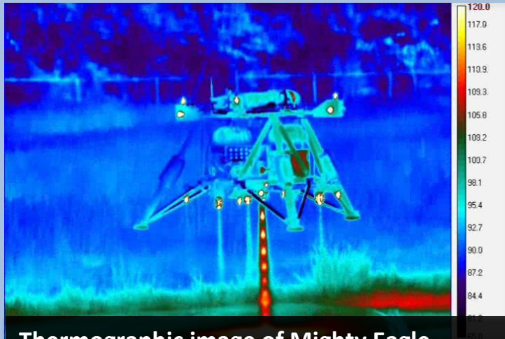
Thermographic image of Mighty Eagle robotic lander demonstration flight
