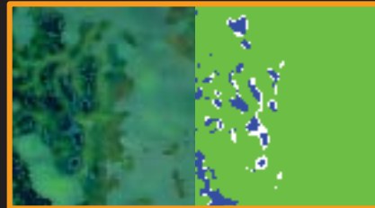
Detect: (L) MODIS imagery of Bang Pla Ma from 20 Jan 2011 (R) Classified surface water extent from MODIS image
