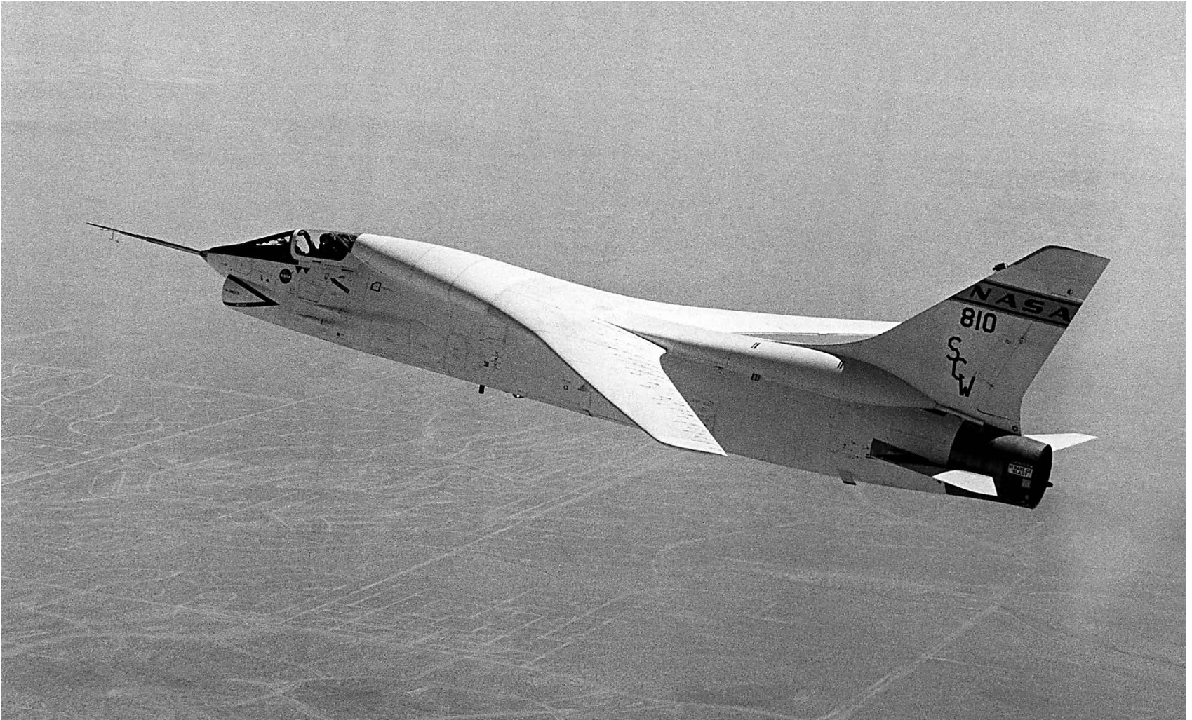
NASA F-8 with Whitcomb Supercritical Wing, 1971
