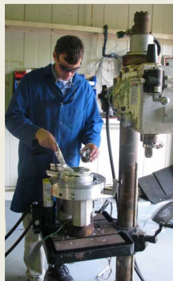
Nike Hercules Igniter Dissection and Chemical Analysis
