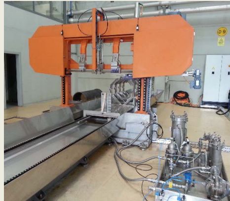
Segmenting 24" rocket motors NEW ~1605 lbs per motor
