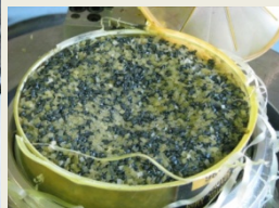
Nike Hercules Igniter Dissection and Chemical Analysis
