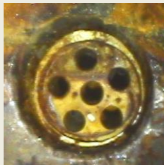
Oxidizer Injector Orifices (Corroded and Restricted)
