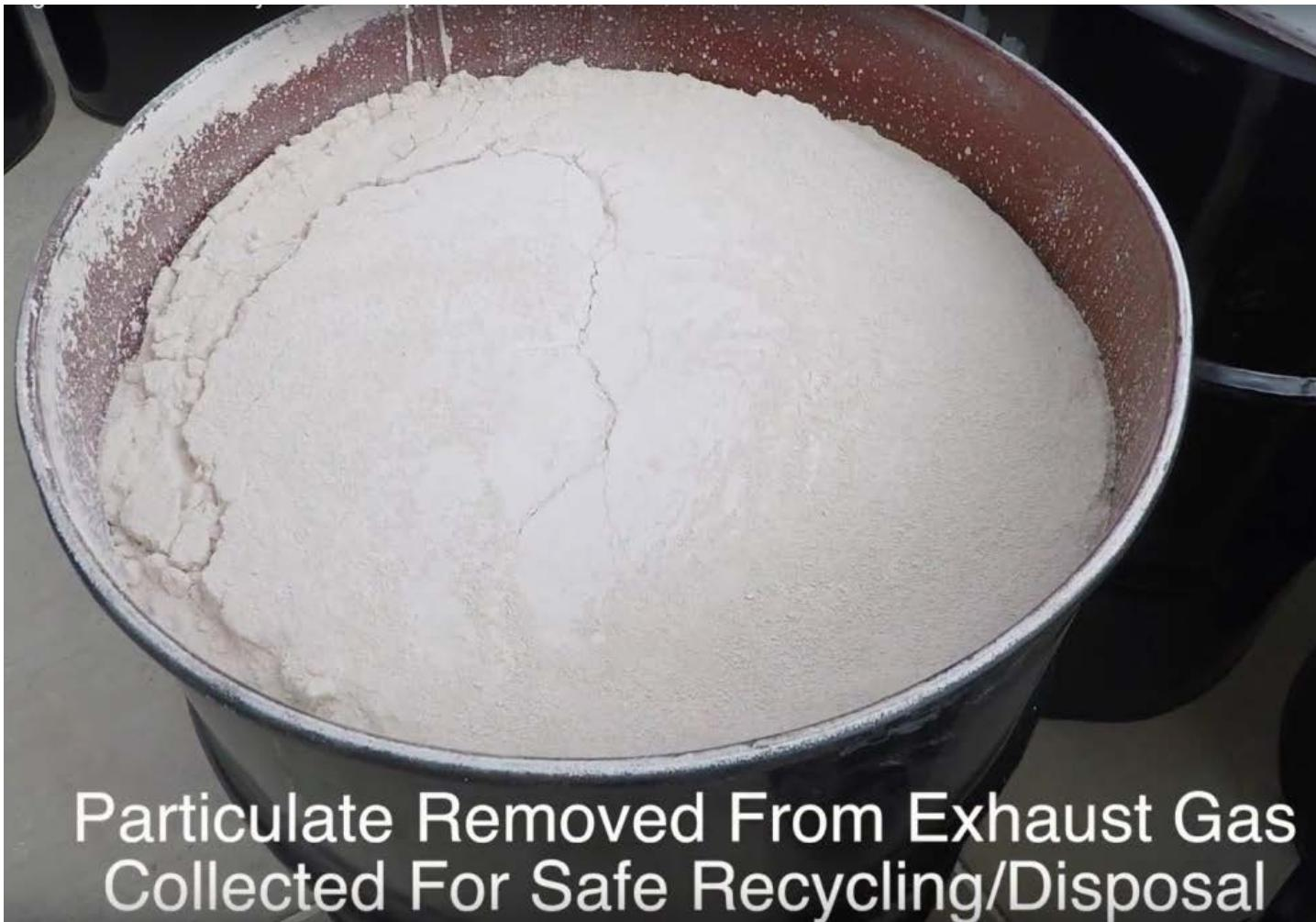
Particulate Removed From Exhaust Gas
