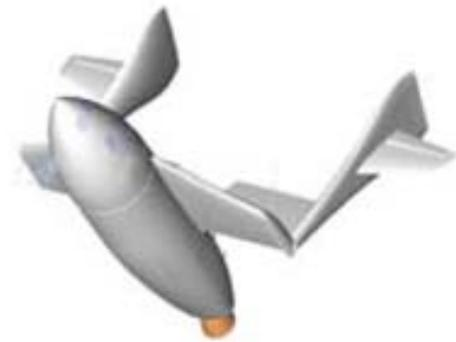
Figure 6<sup>13</sup>. Feathered configuration of SpaceShipOne during reentry.
