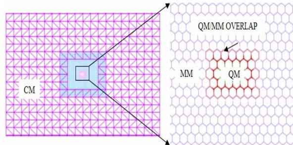
**Figure 1<sup>4</sup>. Coupled QM/MM/CM model of a graphene sheet**
