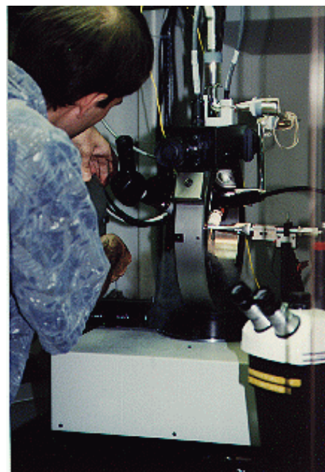
Post-doctoral staff scientist Brian Schick aligns a protein crystal sample on a 4-circle goniostat.
