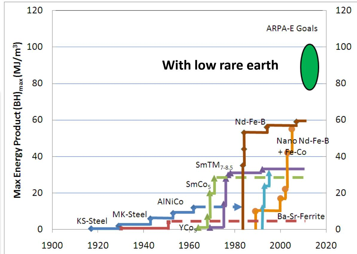
Nanocomposite exchange spring coupled permanent magnets with high energy product and less rare earths
