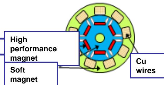
Structure of high efficiency motor
