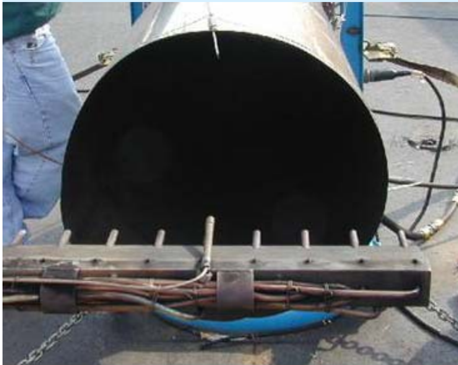
Rake Sampling System At The Outlet Of The JT-12 Jet Engine.
