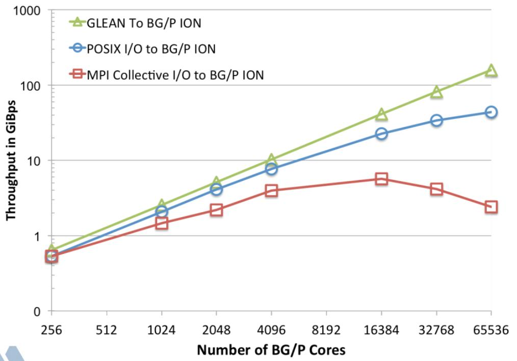
Strong scaling performance for 1GB data movement off ALCF Intrepid Blue Gene/P compute nodes. GLEAN provides 30-fold improvement over POSIX I/O at large scale. Strong scaling is critical as we move towards systems with increased core counts.
