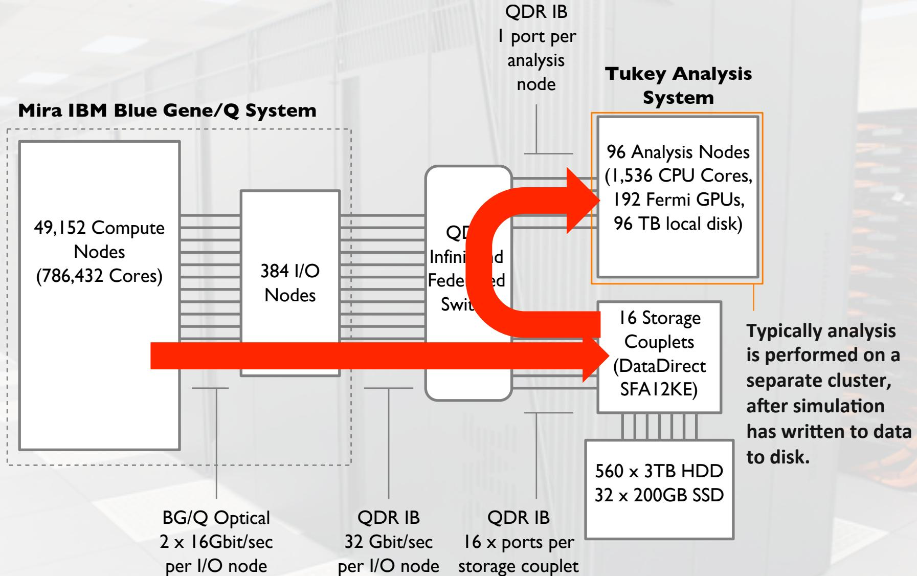
High-level diagram of 10 Pflop IBM Blue Gene/Q system at Argonne Leadership Computing Facility
