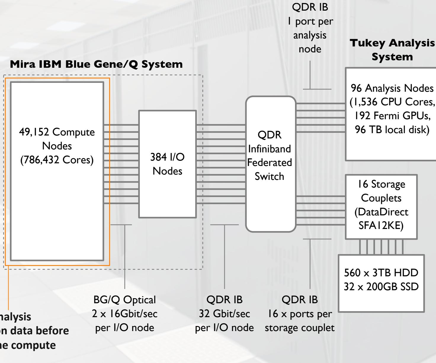
High-level diagram of 10 Pflop IBM Blue Gene/Q system at Argonne Leadership Computing Facility
