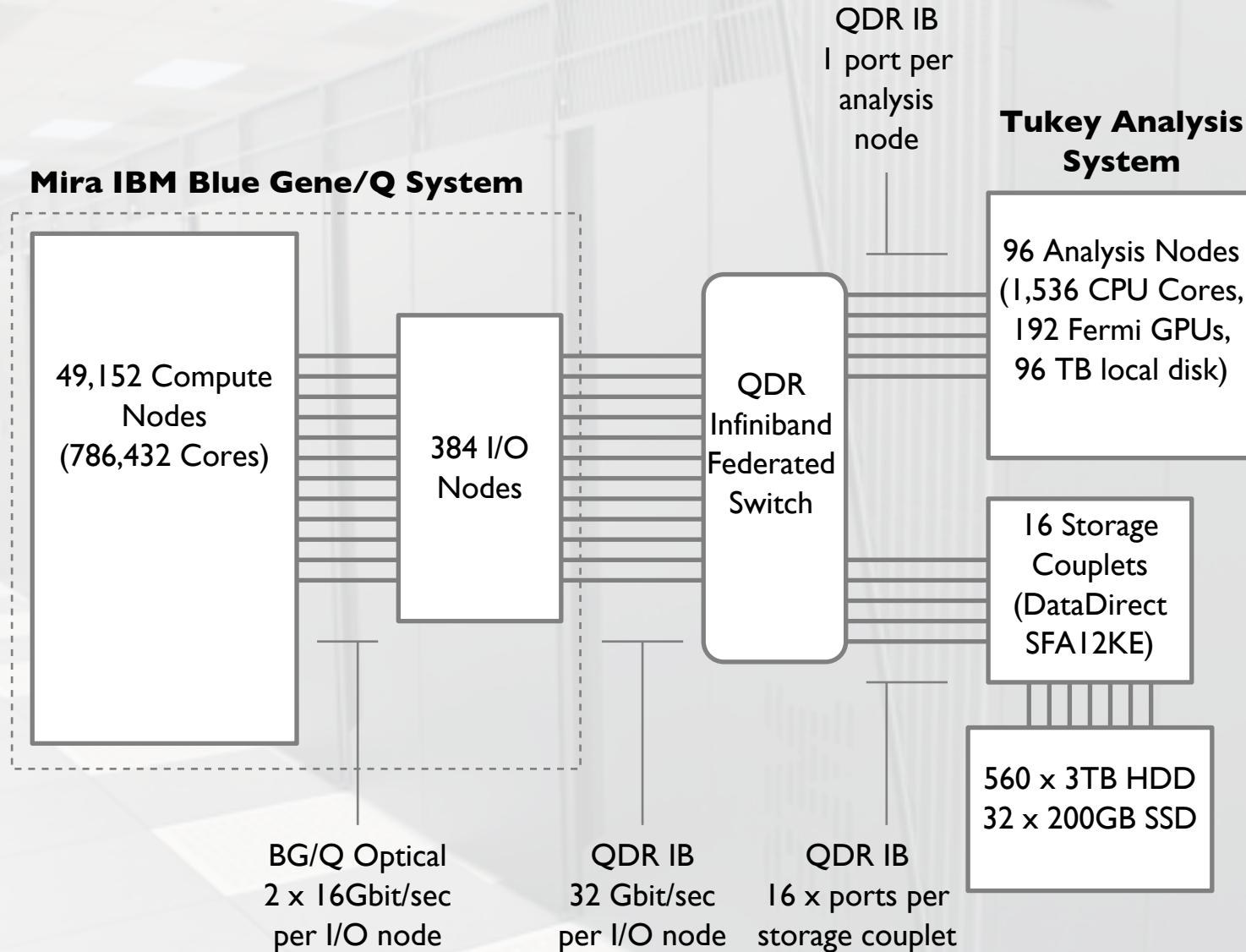
High-level diagram of 10 Pflop IBM Blue Gene/Q system at Argonne Leadership Computing Facility
