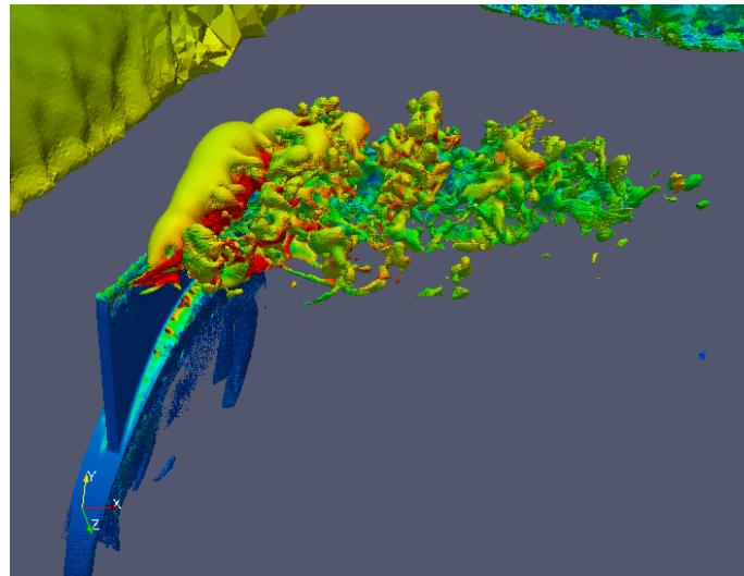
Cut plane through synthetic jet (left) and isosurface of vertical velocity (right) colored by velocity (both for 3.3 billion element mesh). Analysis performed with ParaView.
