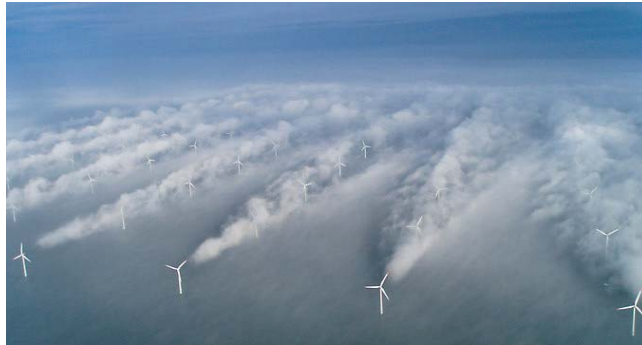
Figure 1. Horns Rev Offshore Wind Farm, North Sea. Turbulent wakes visible in fog behind front row of turbines.
