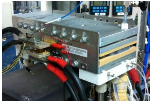
Performance testing of GM Stack for UUV
