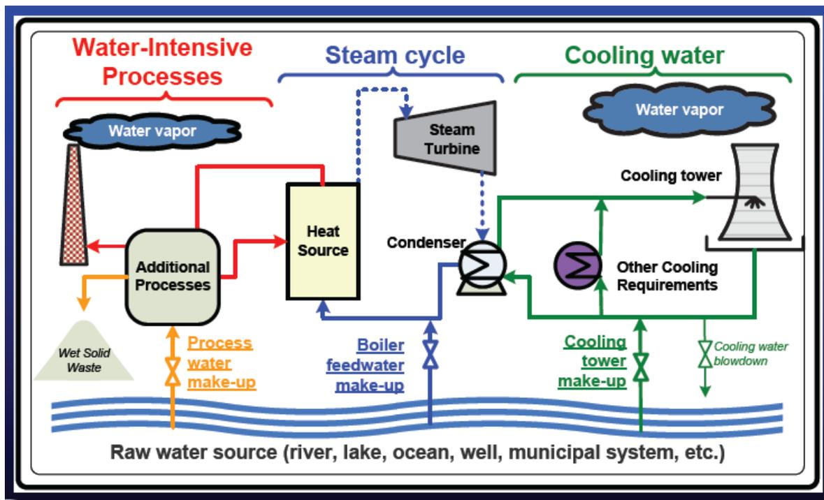
**FIGURE 1** Water use in the thermoelectric industry. SOURCE: Radisav Vidic, University of Pittsburgh, presentation on May 20, 2014, Washington, DC.
