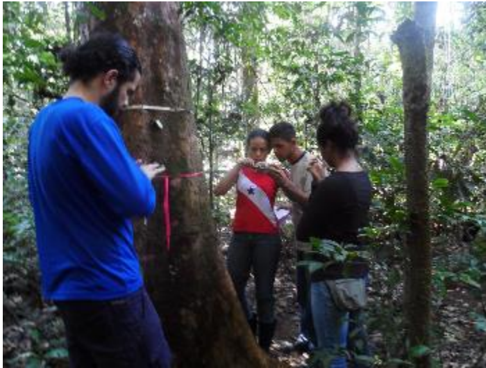
Training of undergraduate students on how to measure stem increment growth in tagged trees, with steel dendrometer bands. (Photo courtesy of Dr. Rosado)
