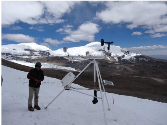
Installation of a weather monitoring station. {Photo courtesy of Dr. Julio Alegria}
