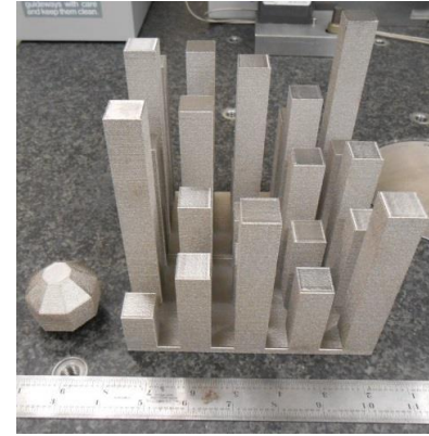
Ti-6Al-4V polyhedron & “Manhattan” artifacts for MPE (maximum permissible error)
