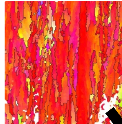
As-built microstructure • Heavily anisotropic
