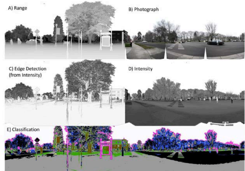
Figure 4. 2D panoramas of scan data. The edge detection (C) and classification in (E) is determined by intensity only. Because computations are done in 2D, they only required milliseconds to complete.
