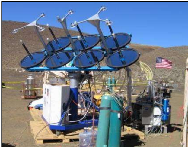
Proof-of-concept ISRU system using concentrated solar energy to produce oxygen from soil being tested in Hawaii
