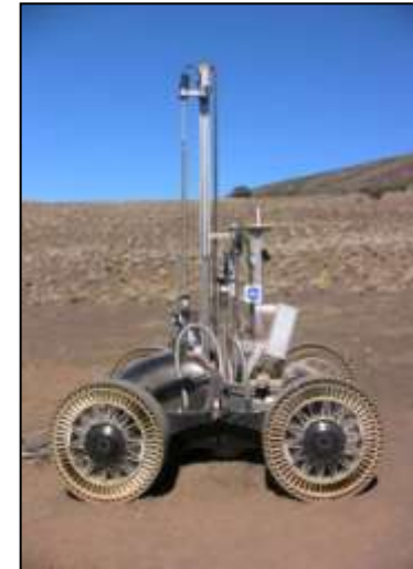
A small rover designed to prospect for ice in lunar craters
