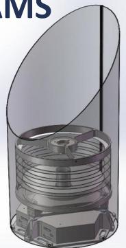
**PolyCam** acquires 1999 RQ36 from 500K km range, refines its ephemeris, and performs high-resolution imaging of the surface
