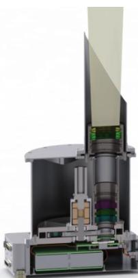
**MapCam** provides narrow angle OpNav, performs filter photometry, maps the surface, and images the sample site
