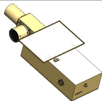
**OVIRS** maps the reflectance albedo and spectral properties from 0.4 – 4.3  $\mu\text{m}$
