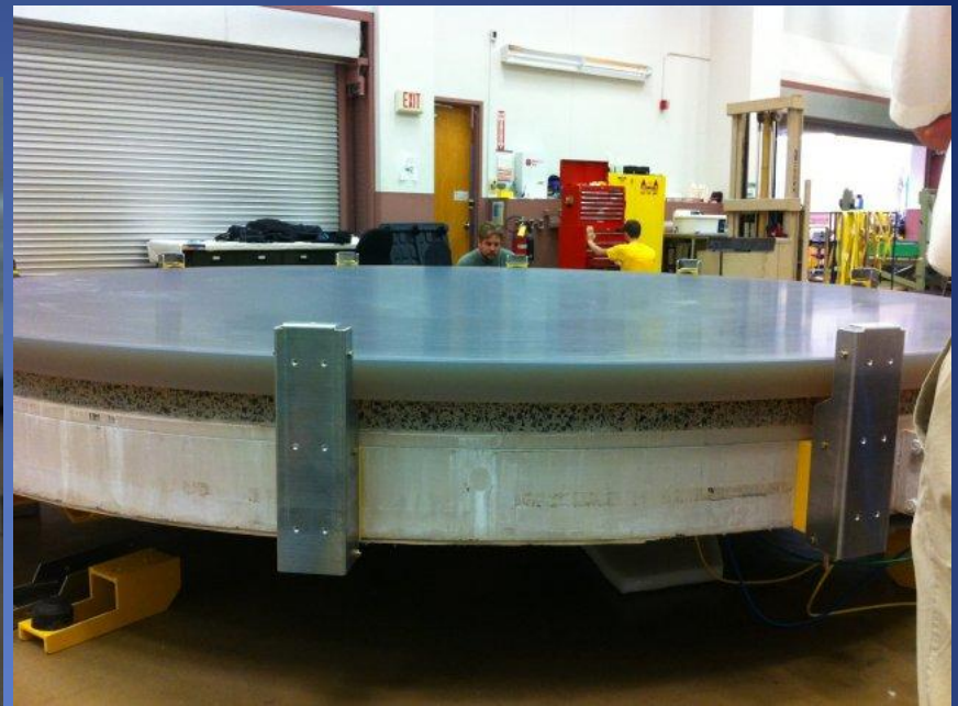
The ATST ± primary mirror commissioning blank, fully exposed, on its support structure being examined by technical staff from Large Optics Shop at the College of Optical Sciences, University of Arizona.
