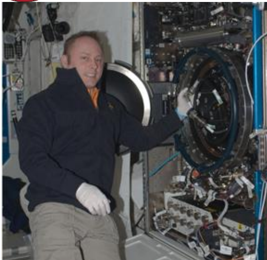
Astronaut Mike Fincke completing install of the CIR/MDCA insert prior to CIR activation in January 2009.
