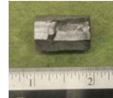
7-hole W-UO 2 in CFEET and post testing up to 2500 C
