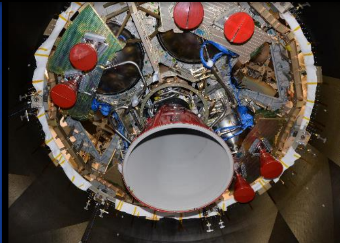
Orbital Maneuvering Engine on the ESM STA at Glenn Research Center Plum Brook Station in Ohio
