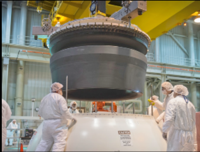
Nozzle installation into the aft booster segment for QM-2
