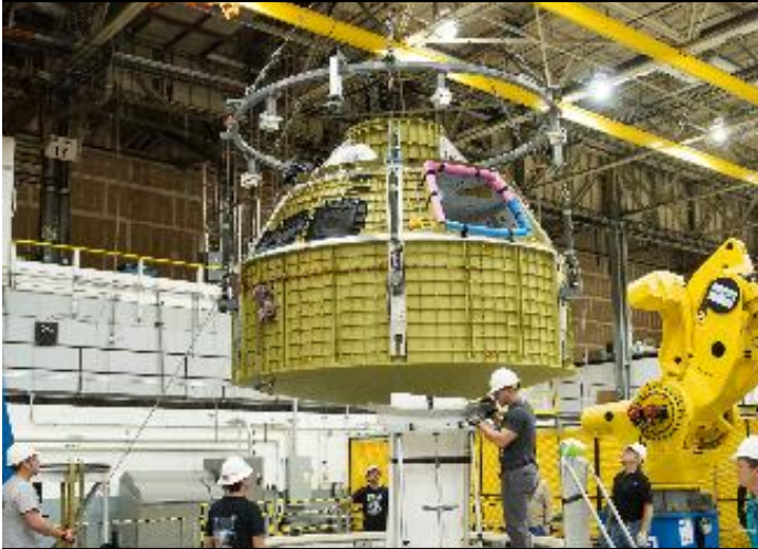
Orion EM-1 crew module pressure vessel welding is completed at Michoud Assembly Facility in New Orleans
