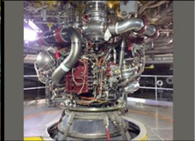
RS-25 flight engine 2059 installed for testing at Stennis Space Center
