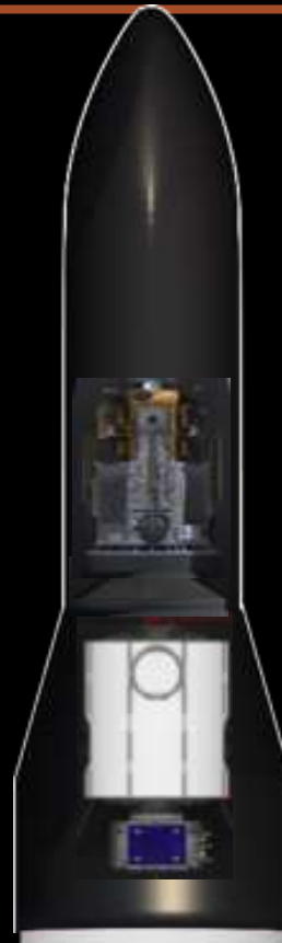
5m fairing w/robotic lunar lander & short- duration hab module
