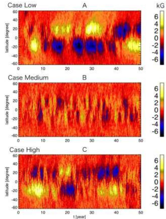
Visualization of magnetic field at base of simulation domain as function of time “butterfly diagram”. The low and high resolution cases (A & C) show a similar coherence whereas the coherence is lost at intermediate resolution (B). (From Hotta et al. 2015, Science 351, 1427).
