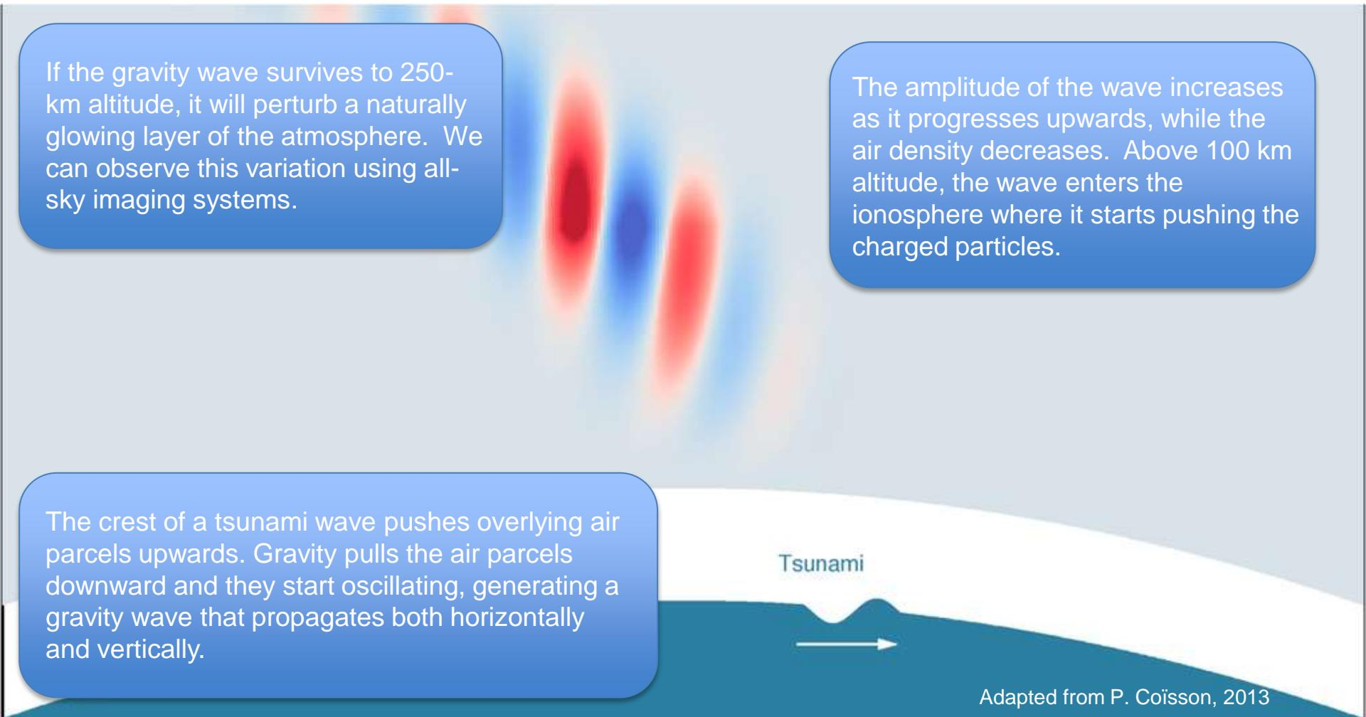
If the gravity wave survives to 250-km altitude, it will perturb a naturally glowing layer of the atmosphere. We can observe this variation using all-sky imaging systems.
