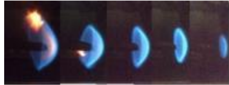
Above: PMMA rod quench sequence in microgravity; Below: Side view of concurrent flame spread
