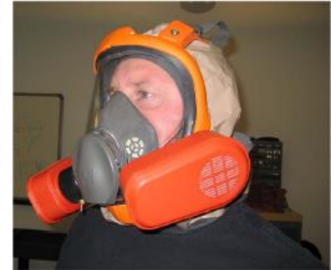
Cartridge is 8 cm wide; sorbent bed is 3 cm deep.
