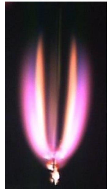
Above: PMMA rod quench sequence in microgravity; Below: Side view of concurrent flame spread
