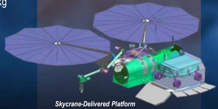
Skycrane-Delivered Platform Concept Packaged in MSL 4.5m Aeroshell
