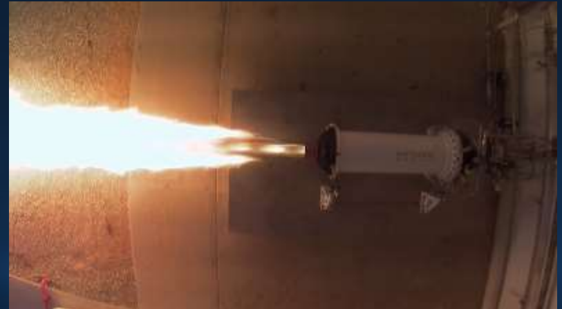
Full-scale hybrid motor test at Whittinghill Aerospace
