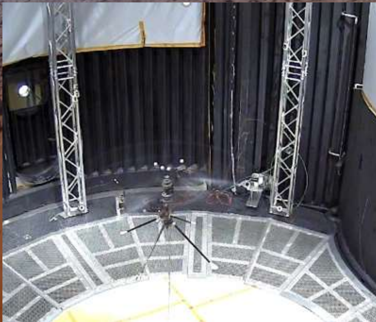
Full-scale free flight testing in JPL Space Simulator
