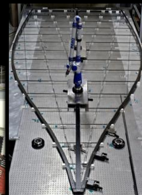
Fabricating the petals to high accuracy (S-4)
