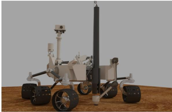
**Figure 2:** WATSON drill with integrated Mars2020 Sherlock instrument could be used to penetrate 1 km depth.
