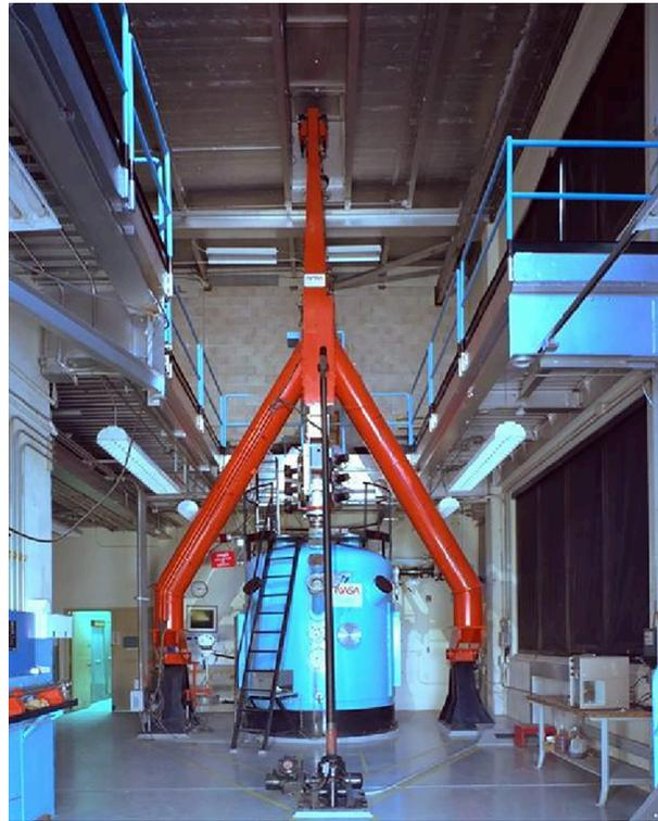
**Figure 2.** The Ames Vertical Gun Range (AVGR) is typically used to simulate high-speed, celestial body impacts on a small scale, and recently it has been adapted to simulate plumes emanating from icy moons [33].
