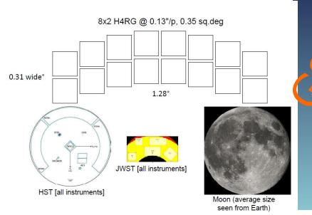
Potential Payload Overview: - 2 wide field instruments 2 small, finer sampled instruments
