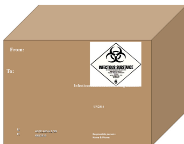
FIGURE: 17-4: Sample Box of infectious substances in Category A Source: IATA Guidelines 2011
