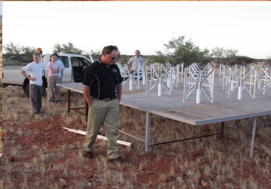
Early prototype of MWA tile
